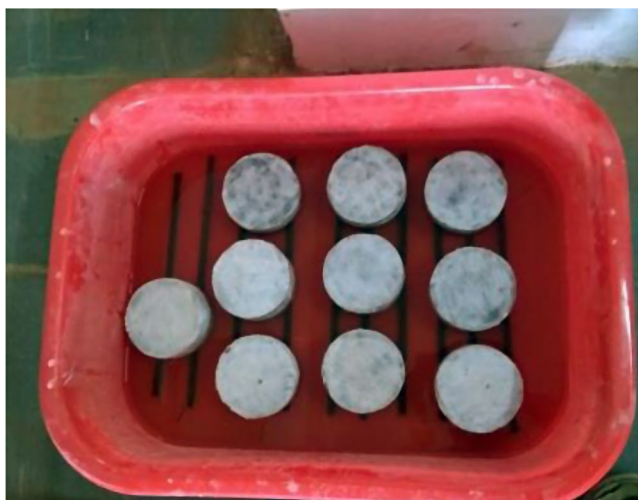
Fig. 6 Experimental photo graph of sorptivity test
